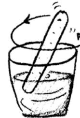
3. Mix equal parts resin and hardener in cup and stir thoroughly.
