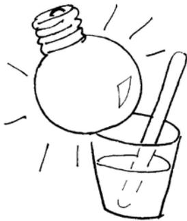
Accurately mix resin 'by eye' and place under lamp to speed up drying.
